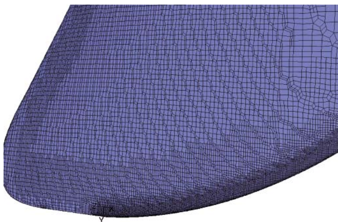
Fig. 2. Computational grid used in Fluent in the tip region of the hydrofoil
