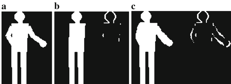
Fig. 11 Hierarchical matching of 3D model to 2D observation of human body: a sample pose, b 3D model posed by first run (high hierarchy) and the difference between pose and model shape, c 3D model posed by second run (lower hierarchy) and the difference between pose and model shape
