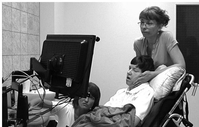
Fig. 4. The Cyber-Eye monitor equipped with a special arm used during the experiment
