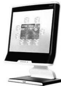
Fig. 1. Tobii T60 – eye-gaze tracking system.
