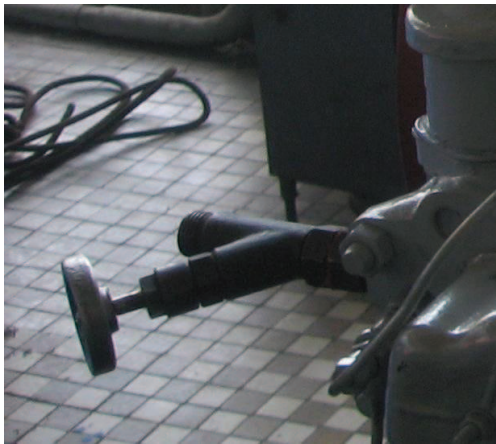
Fig. 2 Indicator valve installed in a place of holder of ignition paper (a) an electronic indicator PREMETS C on a laboratory stand (b)
