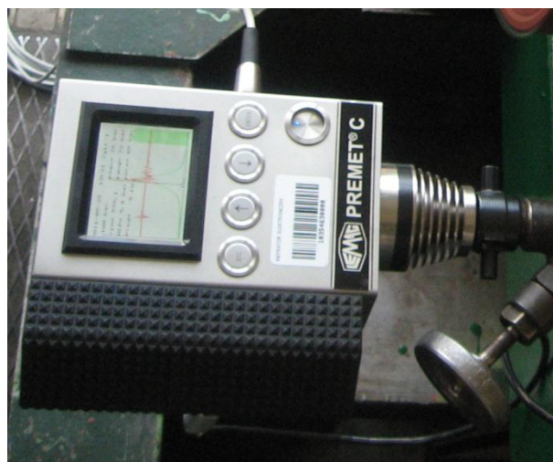
Fig. 3 Electronic indicator LEMAG PREMETS® C
