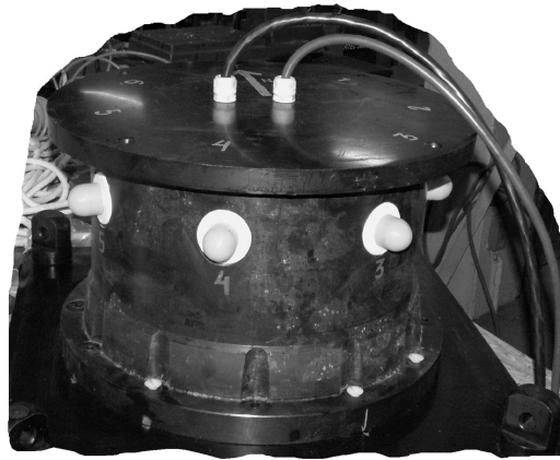
Fig. 4. Photo of the measuring capsule containing six electric field sensors
