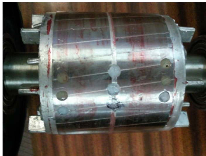
Figure 3: Broken rotor bars and central end ring.
