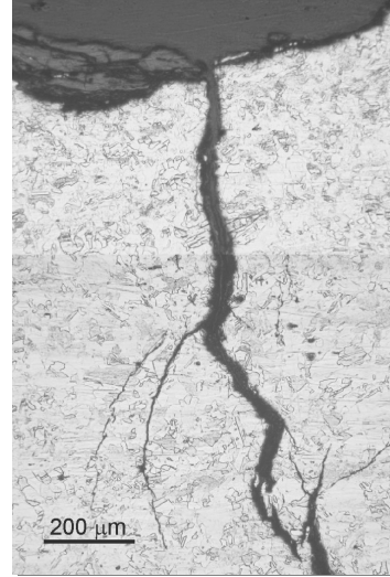
Fig. 12. Transgranular propagation of stress corrosion crack through the pipe wall with characteristic branching
