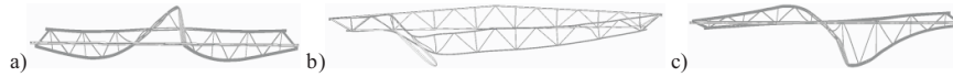
Figure 10 Deformation of the truss after limit load for truss with braces of stiffness 40 kN/m a) 7 braces, imperfection Fig. 6a (a view from the top), b) 7 braces, imperfection Fig. 6b, c) 3 braces, imperfection Fig. 6d (a view from the top)
