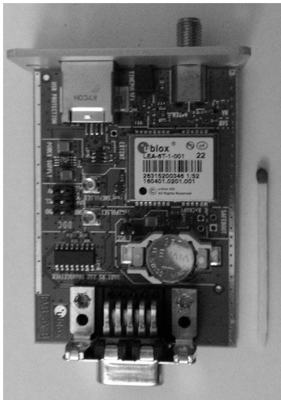
Figure 1. u-blox LEA-6T mounted on the printed circuit board.
