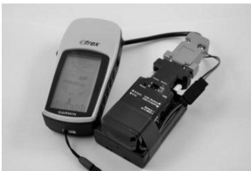
Fig.3. eTrex DGPS used in “Voice Maps” tests [9].
