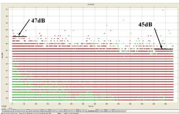
Fig. 7. The change of AE amplitude [dB] at moment of the strain hardening – 10. test piece
