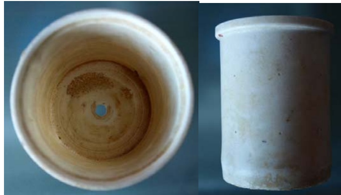
Fig. 4. Electrolytic cell for slow strain rate test
