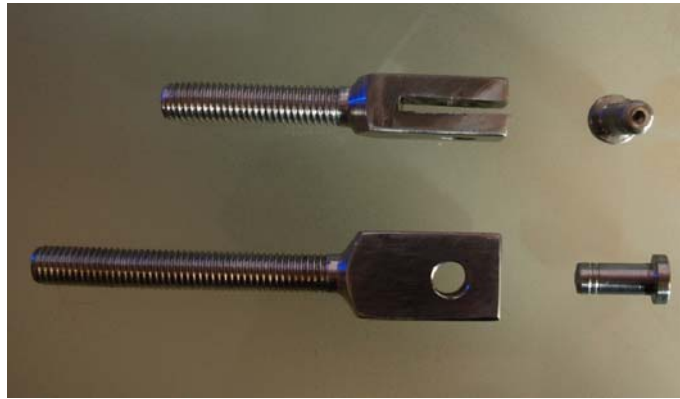
Fig. 3. Clamps fixing the specimens
