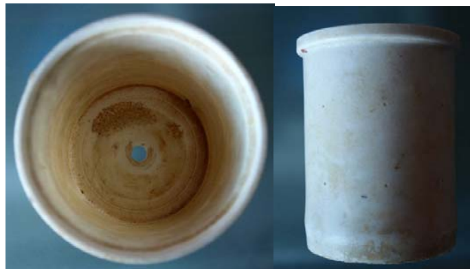
Fig. 4. Electrolytic cell for slow strain rate test
