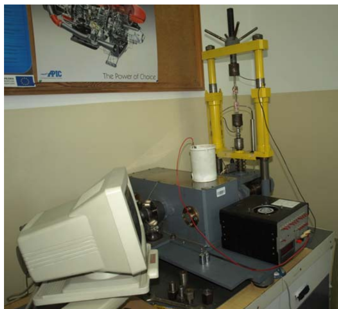
Fig. 2. Equipment for slow strain rate tests
