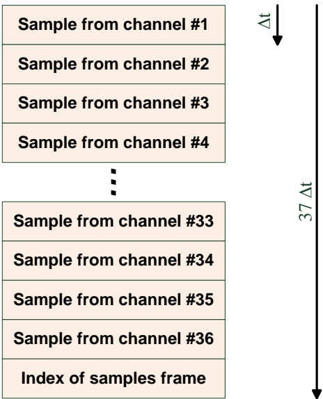
Fig.3. Diagram of sampled measurement data transmission's single frame.
