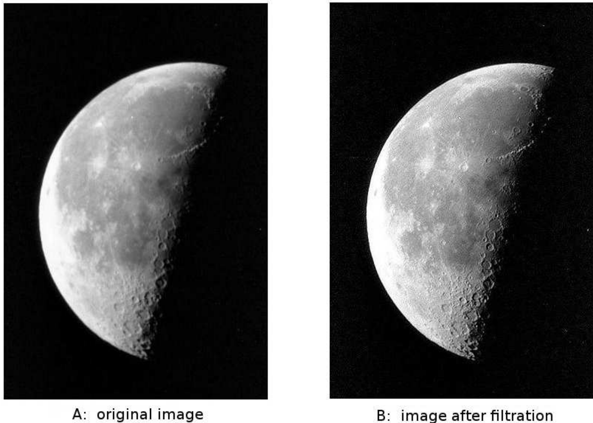
Fig. 5. The result of using a two-dimensional image detailed-emphasis filter. (A) – original image, (B) – image after filtering.
