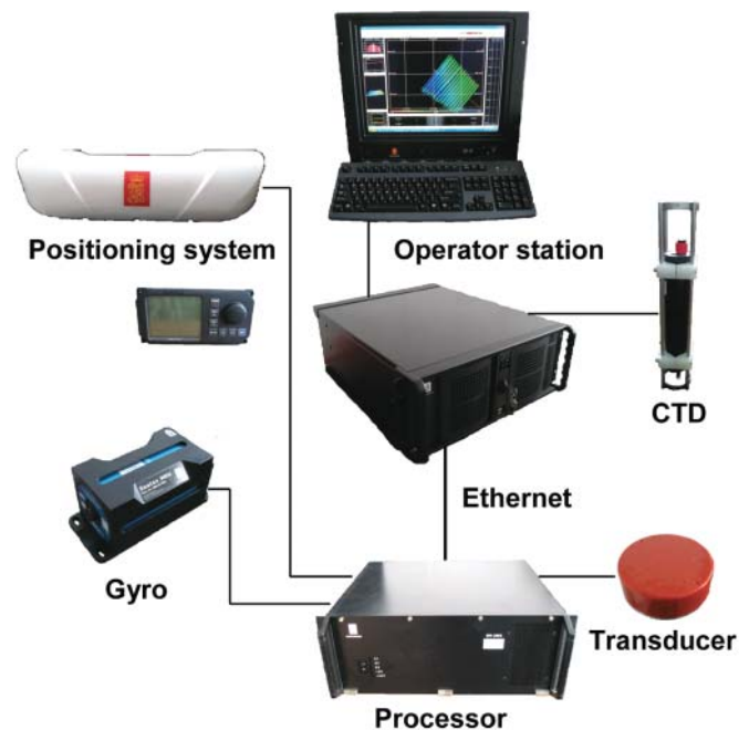
Fig. 1. The overview of multibeam sonar system structure
