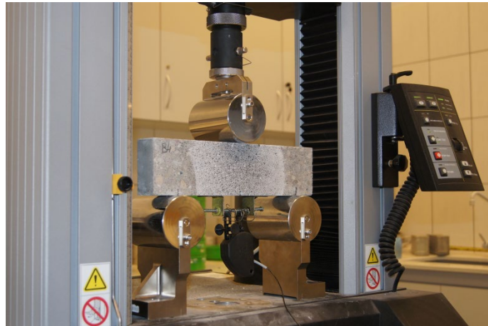
Fig.1: Concrete small-size beam in servo testing machine
