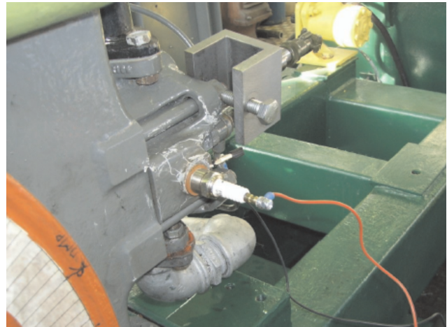
Fig. 4. Langmuir probe mounted in the cylinder of a Farryman Diesel D10 engine
