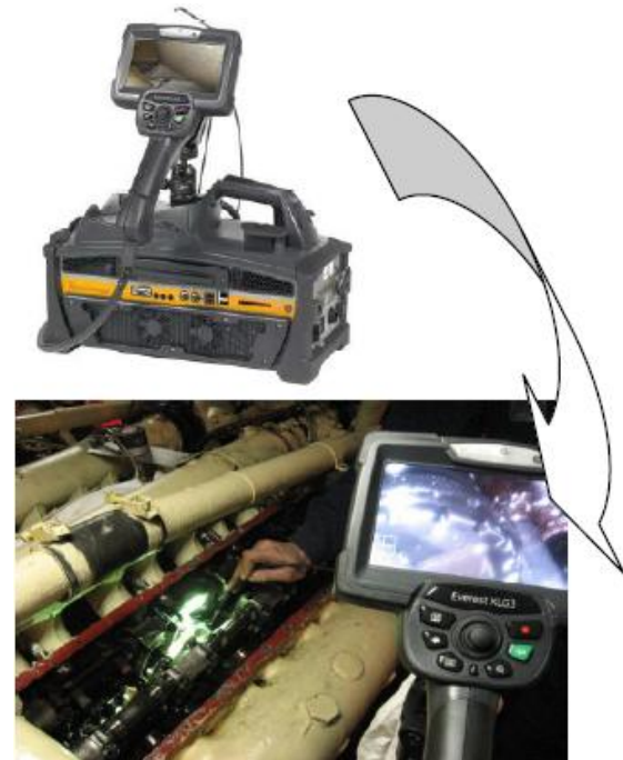
Fig. 3. EVEREST measuring videoendoscope XLG3: general view, b) magnification of the panoramic LCD projector
