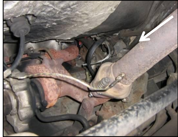
Fig. 3.6. The example of exhaust thermometer montage
