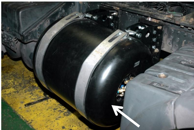
Fig. 3.3. The additional LPG tank in the tractor
