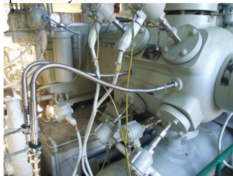
Fig. 6. Pressure sensors mounted in the compressor
