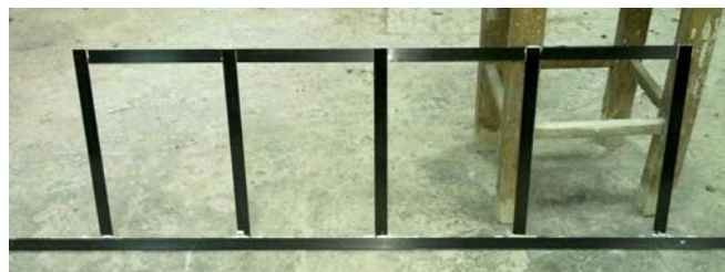
Fig. 3. Reinforcing cage before covering with sand
