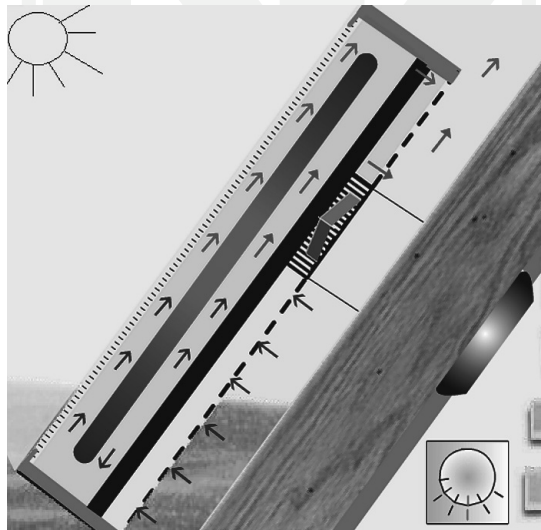
Fig. 4. A working diagram of a SolarVenti sun collector during a cooling cycle [7]
