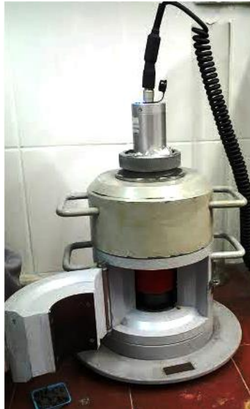
Fig. 3. Scintillation stabilized probe in lead shield used in the research
