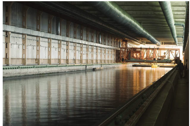
Fig. 9. Model basin (with a mobile towing carriage in the background).
