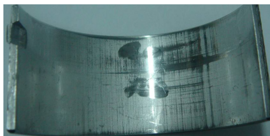
Fig. 6. A view of the bushing surface type MB58 with fatigue damage after test completion [6, 21]
