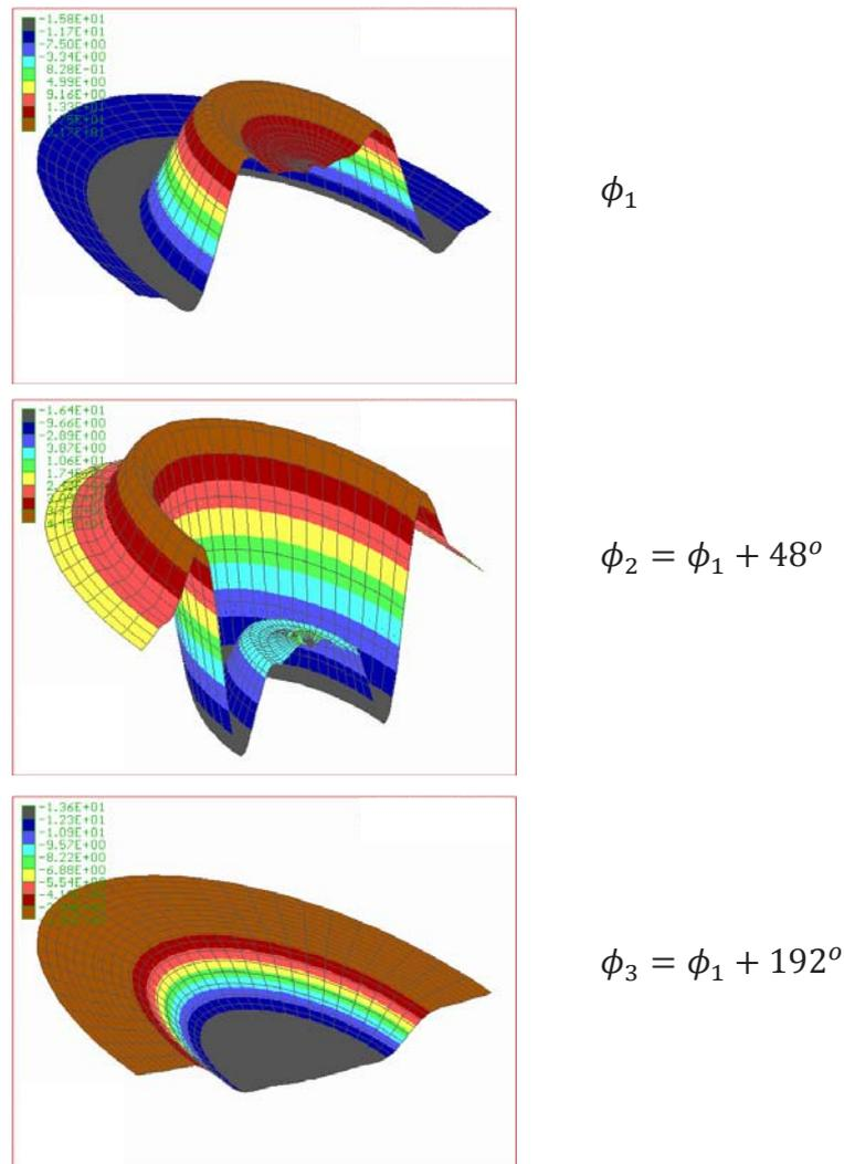
Fig. 9. The temporary pressure distribution on the same plane perpendicular to the beam axis of the circular transducer at different times.
