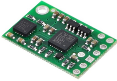
Fig. 1. Tested sensor Pololu IMU9.
