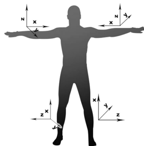
Fig. 1 Location of acceleration sensors on subject's body
