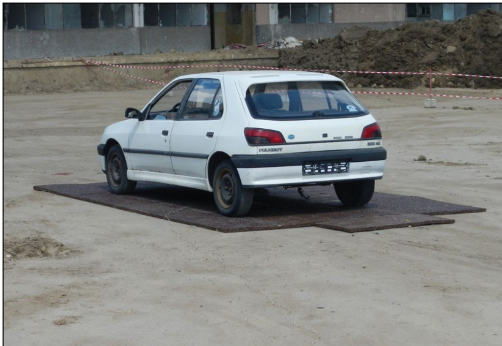
Figure 8. Full scale Fire Test setup
