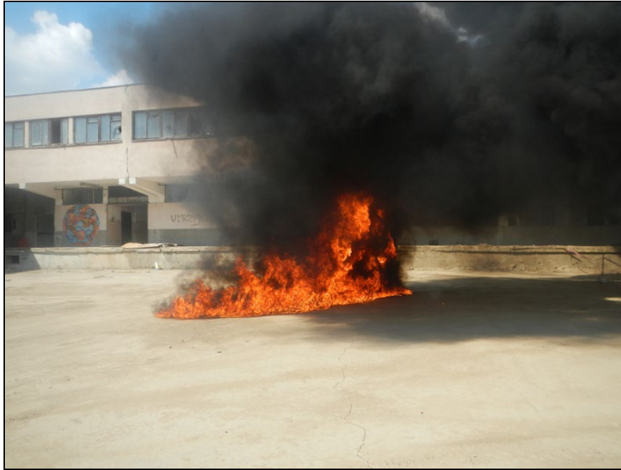
Figure 11. Fire of gasoline spill on the concrete surface (10 seconds after ignition)
