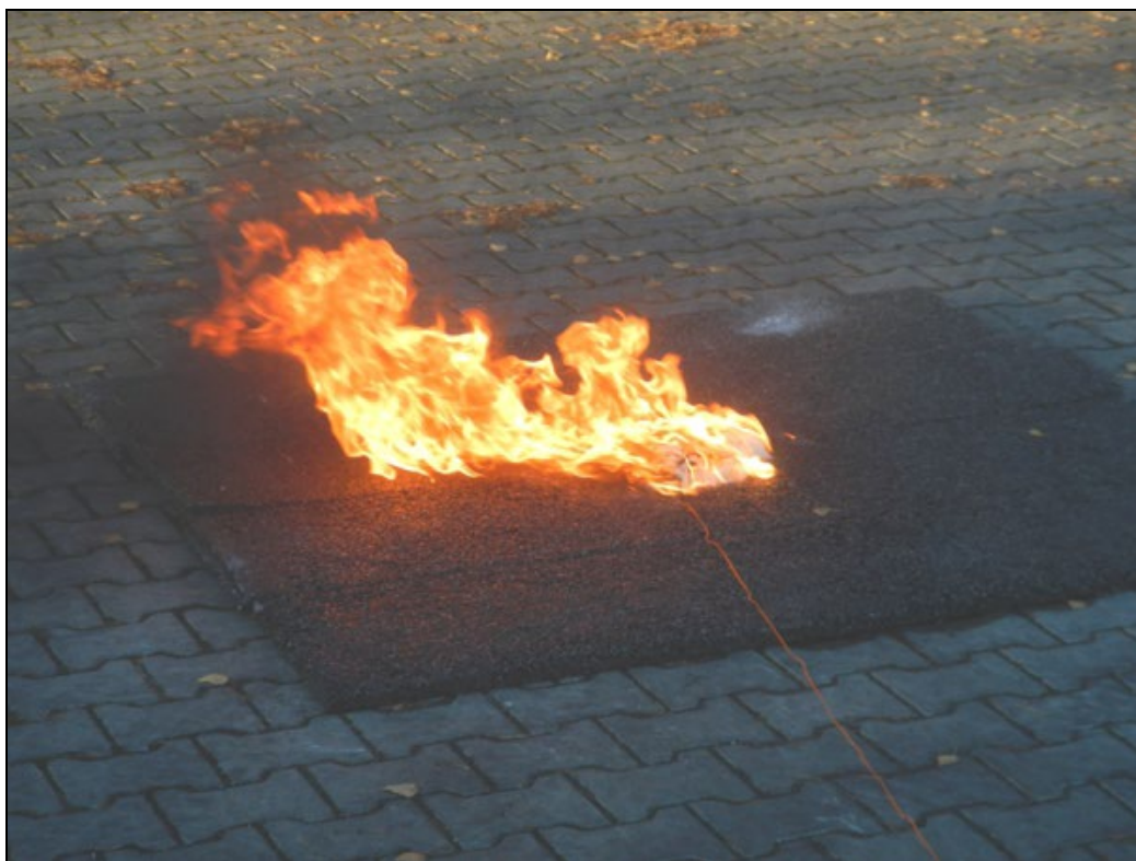
Figure 6. Fire of PERS material 30 seconds after ignition of 2.5 litre of gasoline (strong wind from right side). Heights of the flames is 20 - 30 cm. Cotton wool visible on the right is responsible for most of the flames.
