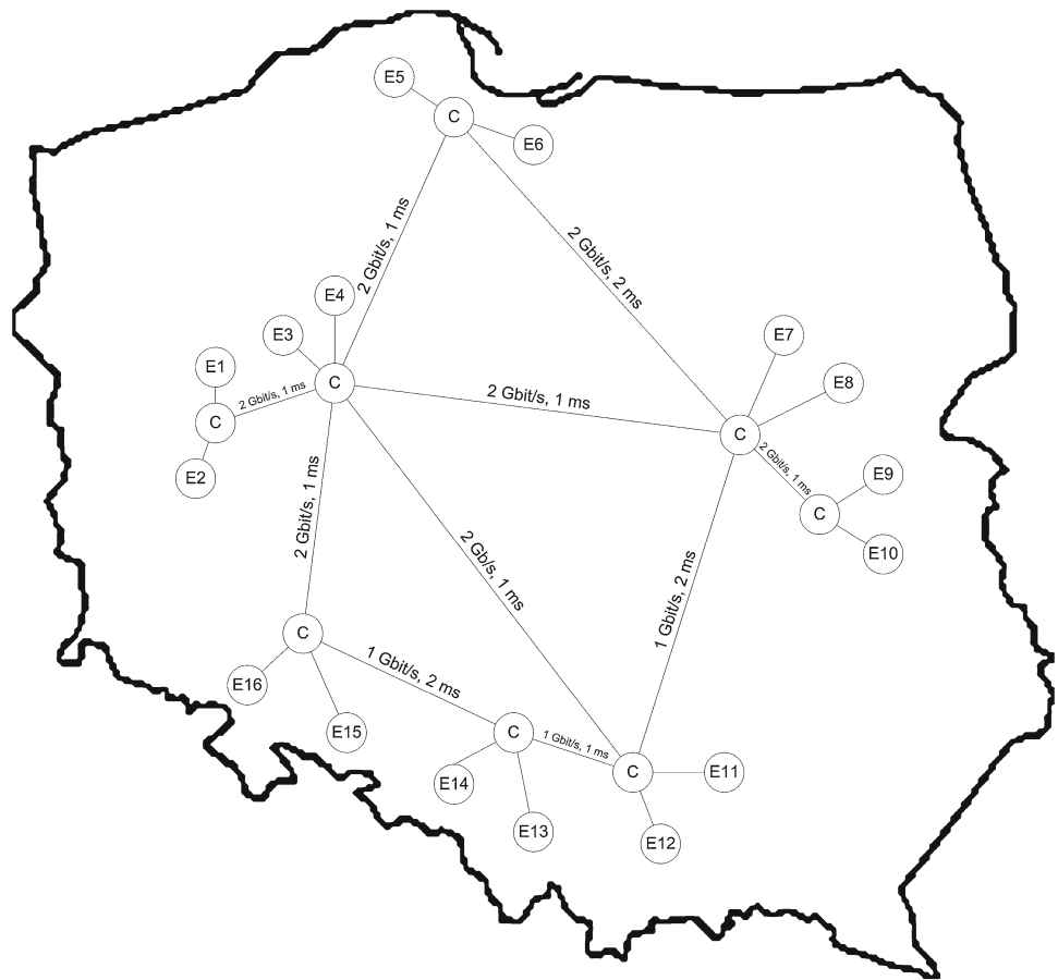
Fig. 1 Example topology of a 24-node Polish network used in computations
