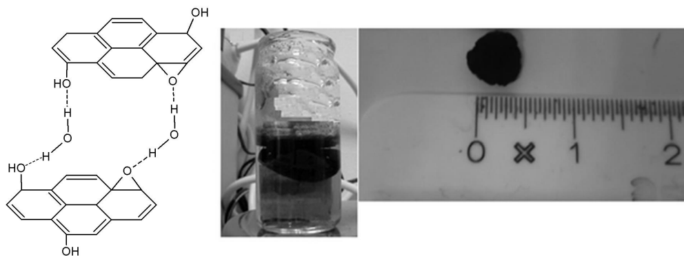
Fig. 4. Left: Formation of hydrogen bonds between rGO sheets. Middle: Graphene hydrogel formed at 95 °C from 2 mg/ml of GO. Right: Aerogel (GA) after drying at room temperature.
