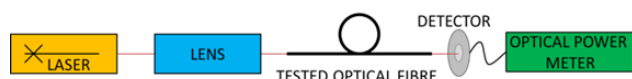
Fig. 1. Scheme of optical power loss setup used for measurement of optical fibres.
