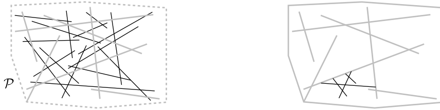
Fig. 32. Adding a virtual simple closed polyline \mathcal{P} allows us to treat the unbounded face as a bounded one.
