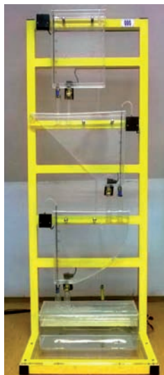
Rys. 1. Kaskada zbiorników Fig. 1. System of cascade tanks
