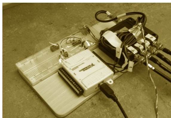
Fig. 5. EMG signals registration system
