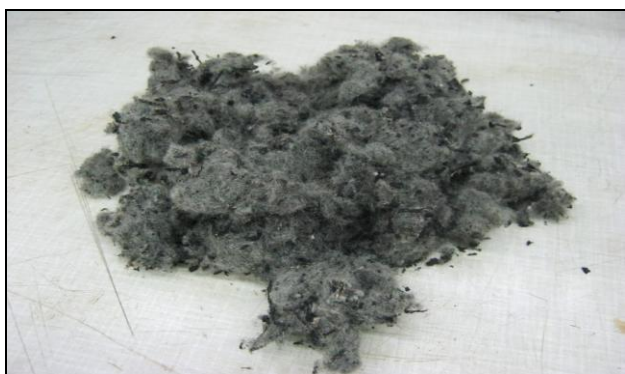
Fig. 1. Recycled textile fiber from used tires.
