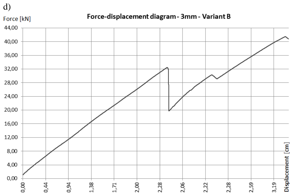
Fig. 5. Force-displacement diagram: a) 2 mm thick sample - Variant A, b) 3 mm thick sample -Variant A, c) 2 mm thick sample -Variant B, d) 3 mm thick sample -Variant B.
