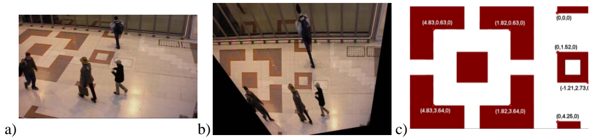
Fig. 3. Image and coordinate space transformations: a) original image, b) after transformation from meters to pixels (every 72 pixels represents 1 meter on the ground), c) ground plan and keypoints coordinates
