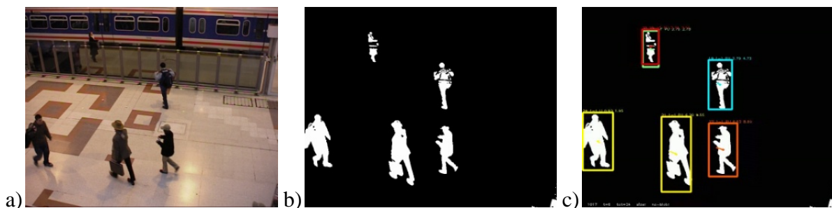
Fig. 2. Object detection and tracking process: a) original frame, b) objects' masks, c) assigned trackers
