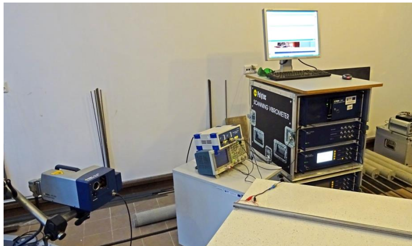
Figure 4. Experimental set-up for wave propagation measurements of ground anchors
