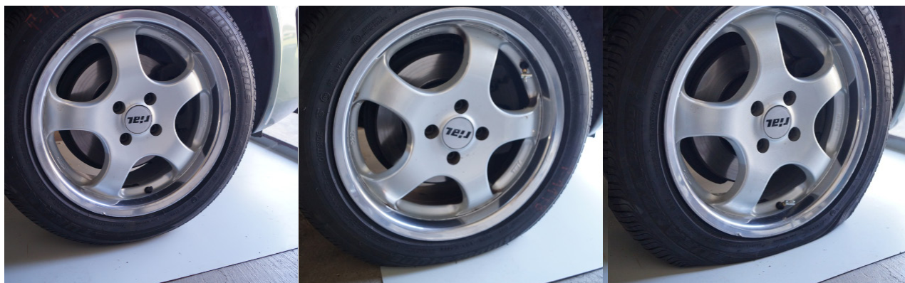
Fig. 2. View of side wall bend for a RUN FLAT tire and a serial tire 205/55R16 Bridgestone. The tire on the left has nominal pressure, the tire in the middle is a depressurized RUN FLAT tire and the tire on the right is a depressurized serial tire (Fig. P. Stryjek, ROSOMAK S.A.)
