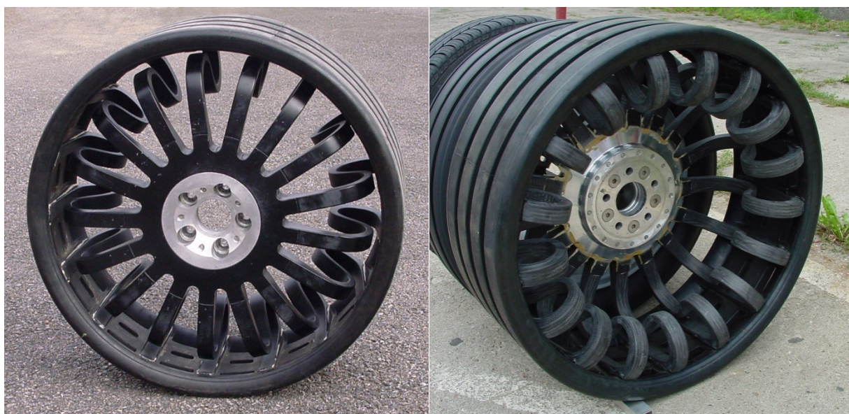
Fig. 6. View of a composite wheel developed in Sweden (Fig. from the archives of the Gdansk University of Technology)
