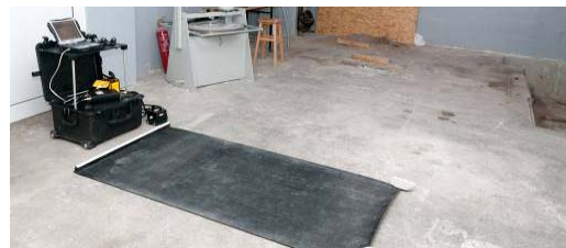
Fig. 4. Ground floor structure during GPR surveys
