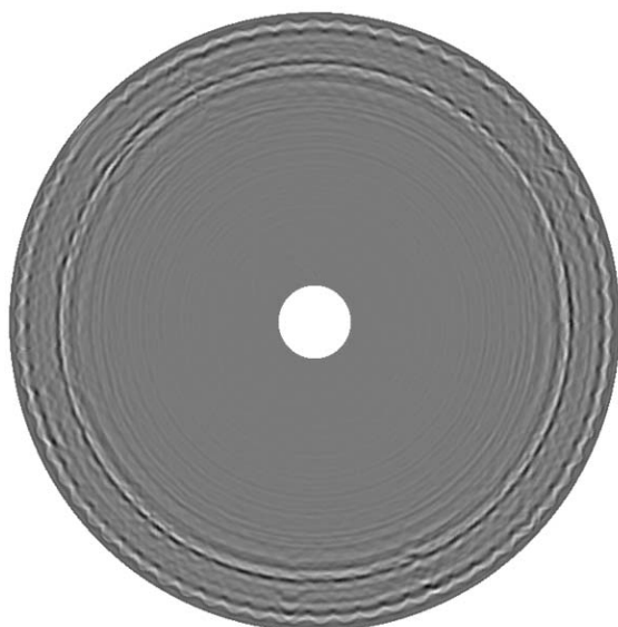
Fig. 13. Curved GPR map of concrete well
