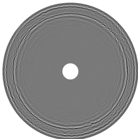
Fig. 13. Curved GPR map of concrete well
