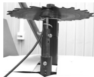
Fig. 3 Laboratory stand for testing circular saws with impact method, where: 1 – contactless inductive sensor, 2 – digital oscilloscope, 3 – NTB with software PicoLog Recorder
