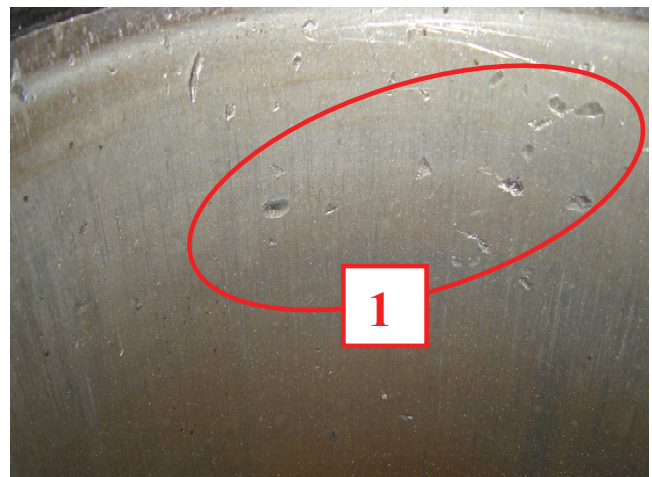
Fig. 6. View of: a) side surfaces of piston 1, excessively worn due to friction (Fig. 5), b) cracked piston rings with losses of material [15, 37]
