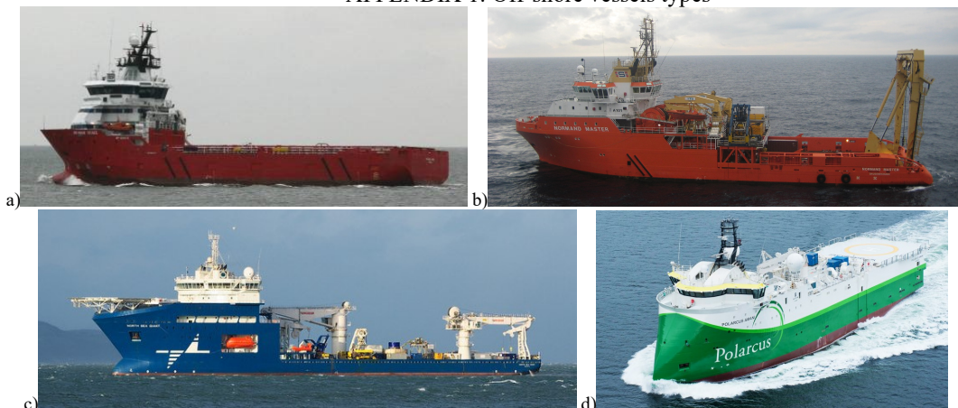
Contours of off-shore vessels: a) Platform Supply Vessel (PSV), b) Anchor Handling Tug Supply Vessel (AHTS), c) Off-shore Construction Vessel (OCV), d) Seismic Support Vessel (SSV).
