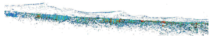
Fig.13. MarLS visualization for the coast fragment with the cloud density parameter of approximately 30 points per m2 for the green colour to approximately 100 points per m2 for the red colour
