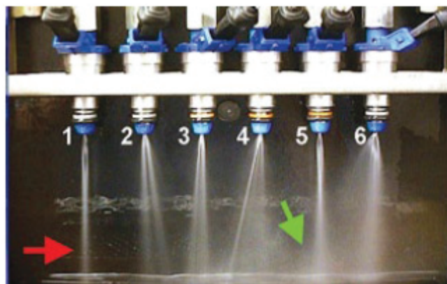
Fig. 7. Pattern of possible disturbances in injectors' operation – full set from the same engine [www.intercars.com.pl]
