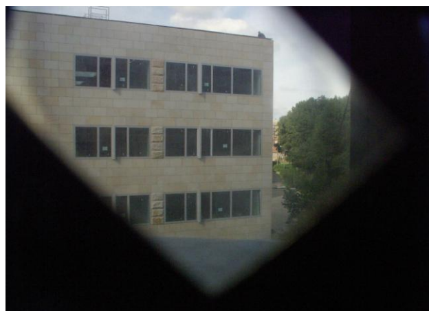
Fig. 3. Building seen through an LCP waveplate placed between crossed polarizers.
