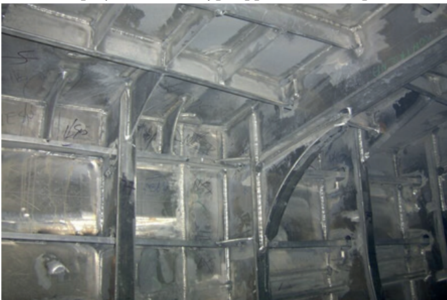
Fig. 1. Typical T-joints in ship structure
